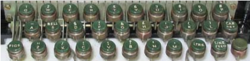
Teleprinter keyboard. It has 32 keys. Each key can produce two characters, the alternate upper character is accessed by first pressing the Figs (figures) key. Access to the lower characters can be restored by pressing the Ltrs (letters) key. Source: Wikipedia.
