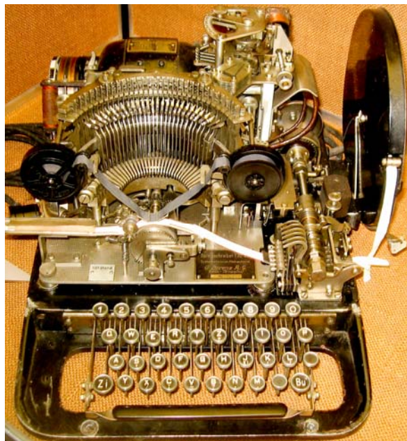
1936 German Lorenz T32 teleprinter (cover removed). It includes a tape reader/punch. Its keyboard has differences from a QWERTY layout for the German language. For example, the QWERTY 'Y' has been replaced with a 'Z'. Source British National Museum of Computing.
