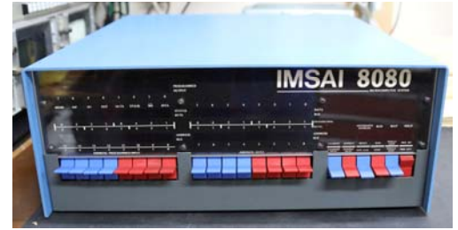
IMSAI 8080 computer, 1975. One of the first small-scale computers initially targeted at hobbyists. It was designed using an Intel 8080 microprocessor and S100 bus architecture. Author's collection.
