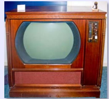
John Staples demonstrated and gave an update on his TK-26 television camera project. He then gave a second talk on challenges and accomplishments in restoring the 30" B&W Dumont Royal Sovereign set. He gave detail on its design including the uncommon use of three I.F. circuits (video, sound, and sync).
