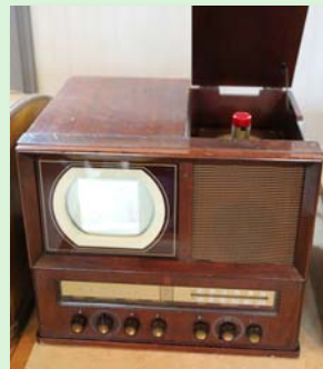
Tom Albrecht compared and contrasted two combination sets in his collection; his smallest, an Airline circa 1952 with a 45 rpm phono, and his largest, a Dumont RA101 Westminster with a 78 rpm phono and a motorized tilt-away CRT that he demonstrated to the group in 2014.
