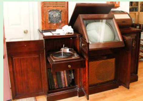
Tom Albrecht compared and contrasted two combination sets in his collection; his smallest, an Airline circa 1952 with a 45 rpm phono, and his largest, a Dumont RA101 Westminster with a 78 rpm phono and a motorized tilt-away CRT that he demonstrated to the group in 2014.
