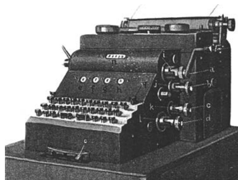
First model of Enigma, the Model A. Source : The Commercial Enigma - Kruh & Deavours
