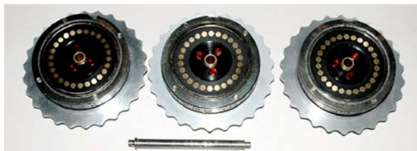
A three-rotor set shown from the side with flat contacts. The thumbwheel is used to turn each rotor for the initial setting. The rod in front is the axle. Source: Enigma Museum.com
