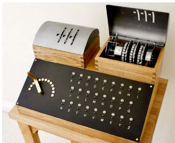
A reproduction of the Cyclometer built by Henry Evans, University of Cambridge. The cyclometer finds permutation cycles for possible solutions of Enigma keys. Two sets of 3 Enigma rotors are mounted in the compartments at top to left and right. The panel has lamps (A-Z) and a rheostat (left) that controls the brightness of the lamps. The intent was to make a faithful reproduction based on the scant information available. Henry Evan explains its operation on Youtube (search for Cyclometer Evans).
