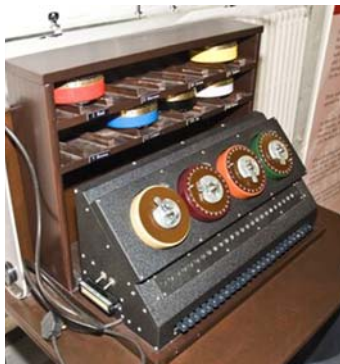
Enigma like device to test the results of a Bombe Stop. Source: The National Museum of Computing.
