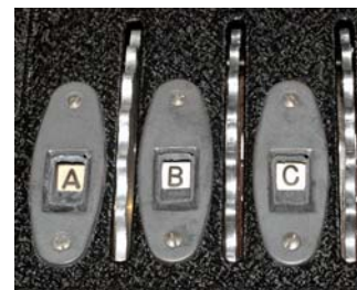
Windows showing rotor values. The rotors advance one at a time like an automobile odometer. The right rotor turns first followed by the middle, then left rotor. A notch on each rotor causes the turnover (i.e. advancement) of the next.
