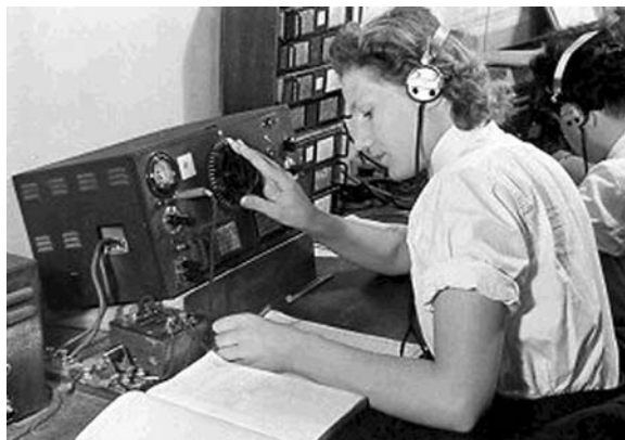
WWII Y-service wireless intercept operator using a National HRO receiver. Source: CryptoMuseum.com
