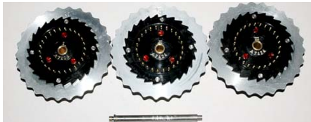
Other side of the three-rotor set showing the contact pin side. The ratchet wheel meshes with a pawl mechanism that advances the rotors like an odometer during operation. Source: Enigma Museum.com
