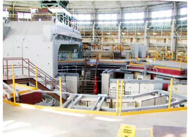
Fig. 11: Berkeley Advanced Light Source Booster Synchrotron in 2015. The inverted U-shaped magnet structure from the 1940s (in grey) was too large to remove and remains there today. (Collection of John Staples)
