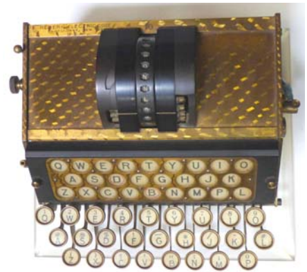
This is an early version of the Hebern encryption machine. It had just one rotor. Later models had 5 rotors that advanced like an odometer. Source: Cipharmachines.com
