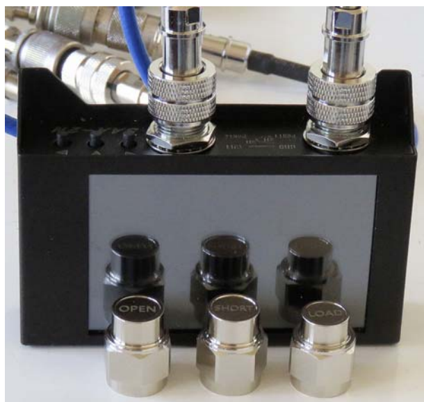
The SAA2N and its calibration standards
