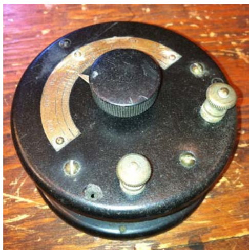
Murdock Variable Condenser (i.e. capacitor).
