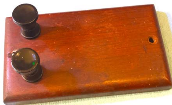
Capacitor shunt for the headphones..
