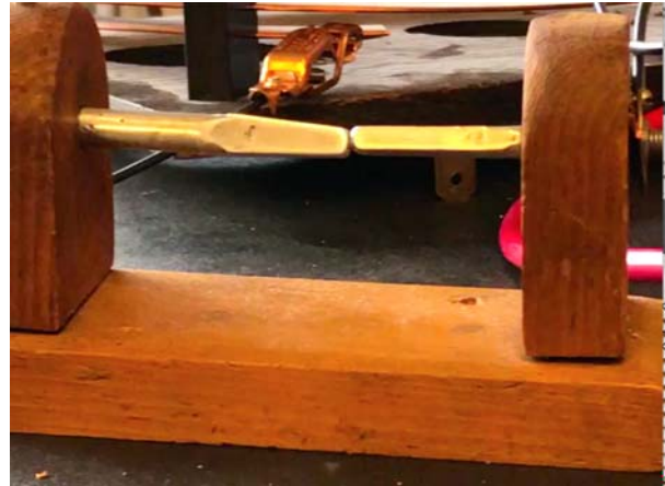
Handmade Zinc Spark Gap.
