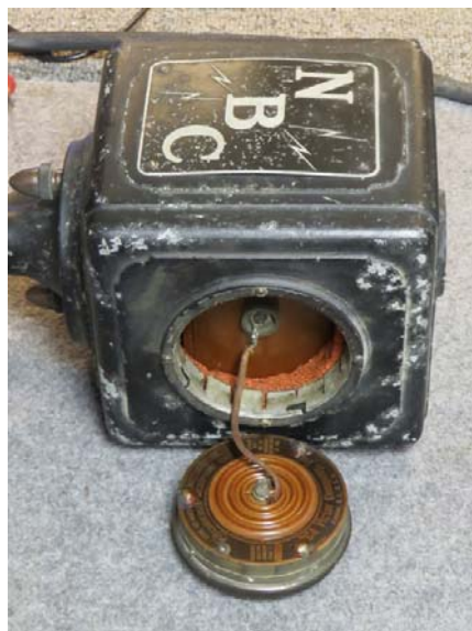
Condenser cartridge removed.
