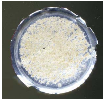
Corroded diaphragm with a hole.
