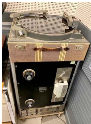
A 16" Presto ET cutting lathe sits atop our Ampex ABR-10 15" station logging recorder.
