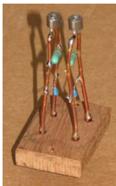
IF transformer for an AA5 built by Robert H. The two halves are positioned to provide space between the inductors for mutual coupling. (Images from the Antique Radio Forum).
