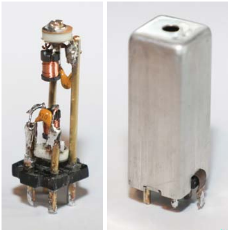
One of the two IF transformer assemblies.
