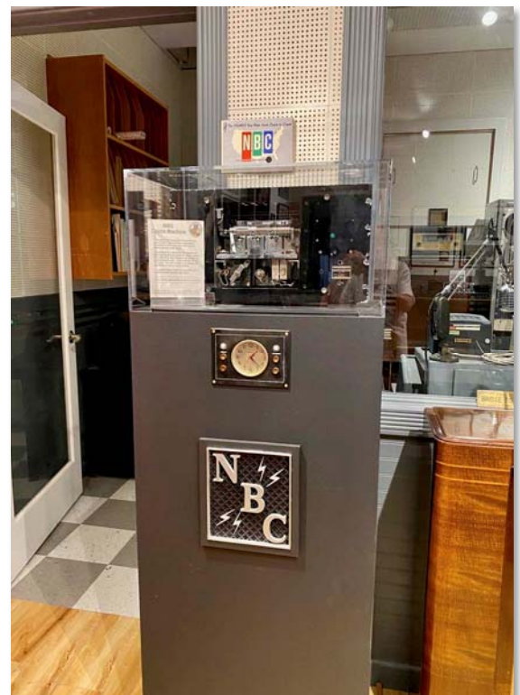
CHRS' NBC/RCA Rangertone chime machine, Serial #002. Used for many years to generate the familiar 3 note tones on the NBC radio network. This unit is from NBC's West Coast 'Radio City' facility at 420 Taylor Street in San Francisco, home of KPO-AM, later becoming KNBC-AM. The chime machine was generously donated by Bill Newbrough and restored by John Staples and John Stuart.
