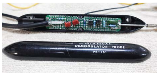
The internals of the active probe I built from John Staples design. I used the casing from an old TV test demodulator probe.
