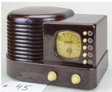
45. Zenith / 5R312 1938; AM band; electrically restored. Has audio input.
