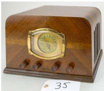
35. Stewart-Warner / 1801 1937/38; AM/SW; electrically restored. Has audio input.
