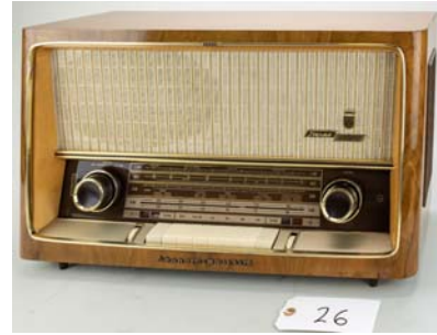
26. Grundig Majestic / 3192U 1961; AM/FM/SW; electrically restored. Has audio input.
