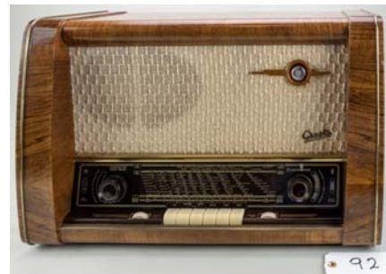
92. Graetz / Super 171W 1953; AM/SW; electrically restored. Has audio input.
