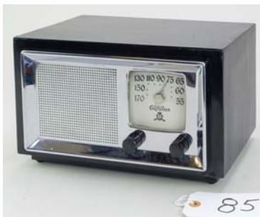
85. Gilfillan / 56B 1946; AM band; electrically restored. Has audio input.
