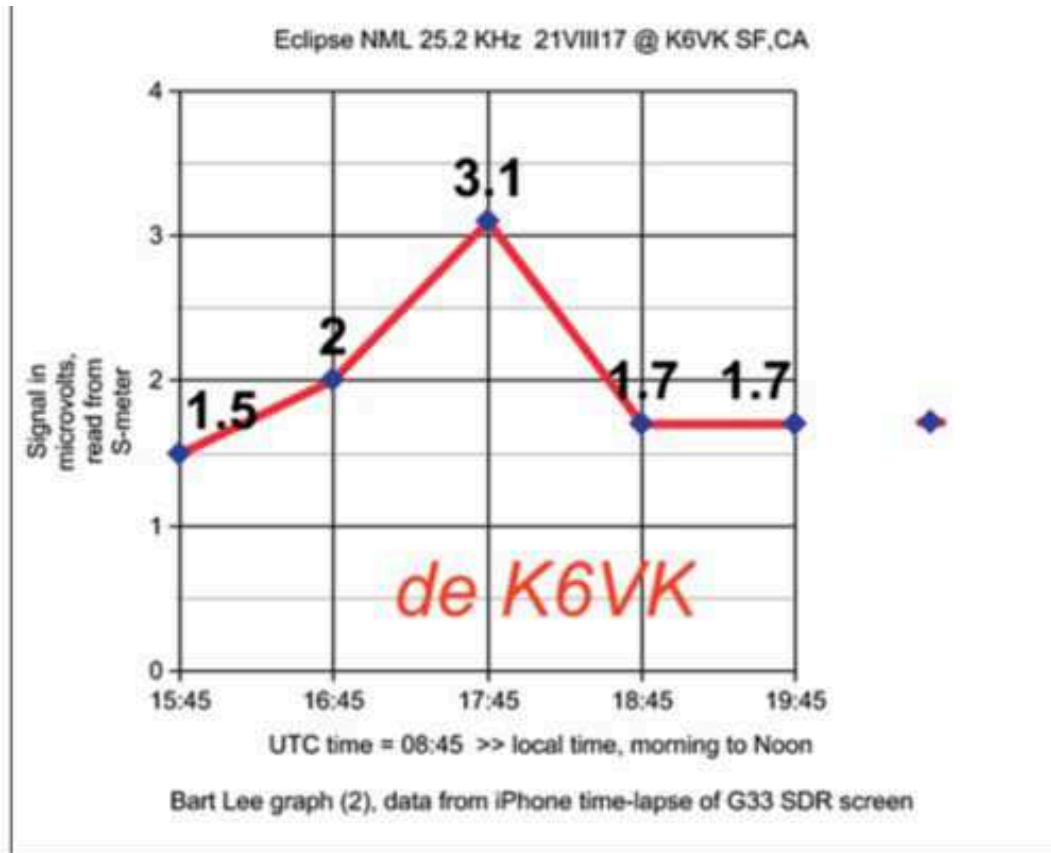
Fig. 46. Graph of increase in VLF station NML (ND) signal strength in California during the eclipse, 6dB+. (Author)
