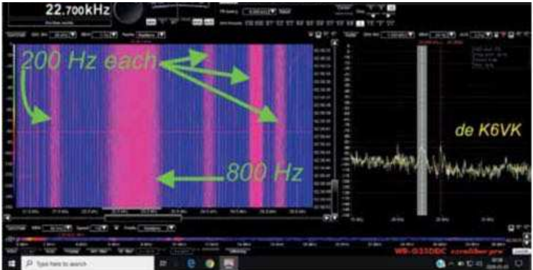
Fig. 38. A strong (32 microvolt), 800 Hz bandwidth MFSK VLF signal appeared at 22.7 kHz on May
