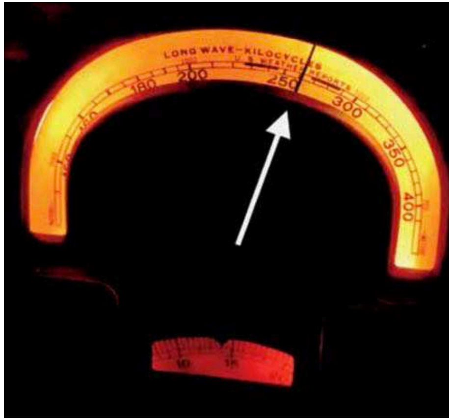
Fig. 25. The dial showing the “Weather Band” around 250 kHz, on a 1936 RCA 10K console radio. (Author’s collection)
