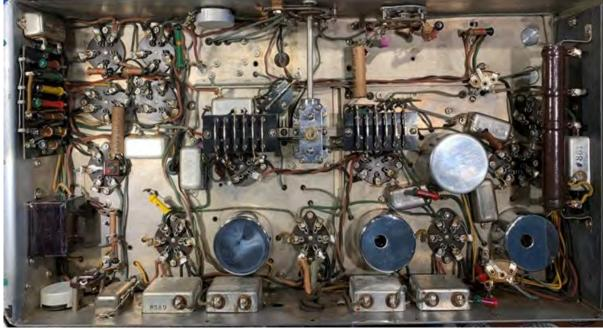
above-chassis can electrolytics were absent, with blanking caps present in the holes in the chassis the electrolytic capacitors would have occupied.
