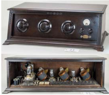
33. Garod / V Neutrodyne Start Bid: $120 1925; AM band. Comes with good 01-A tubes.
