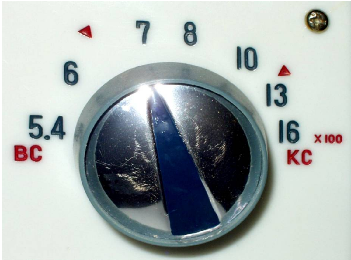
A typical CONELRAD marked dial on a Viscount radio; photo Konrad Brinker on Radiomuseum.org
