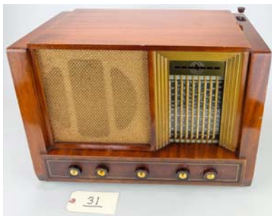
31. Philco / Trans-Ocean 19--?; LW/AM/SW; electrically restored. Has audio input. Euro set?
