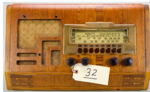
32. Philco / 39-30 1939; AM Band; electrically restored. Has audio input.
