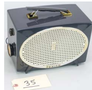
35. Zenith / Y513G 1955; AM Band; electrically restored. Has audio input.
