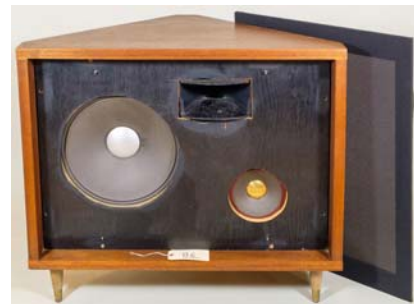
86. JBL, Stephens / 16 ohm working speaker set JBL D-130, JBL 275 w/ H5040 horn, Stephens 80FR 8" driver. JBL 3105 crossover. Generic cabinet.
