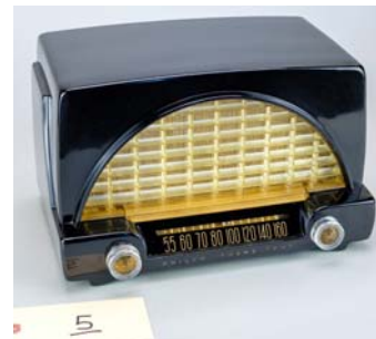
5. Philco / 51-532 1951; AM Band; electrically restored. Has audio input.
