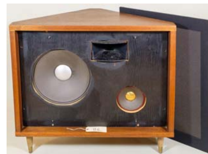
86. JBL, Stephens / 16 ohm speaker set JBL D-130, JBL 275 w/ 90" horn, Stephens 80FR 8" driver. JBL 3105 crossover. Generic enclosure.
