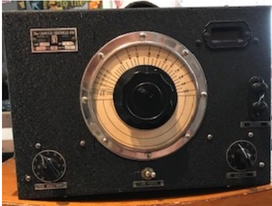
A Beat Frequency Oscillator "79"; Bart Lee Collection and Photo
