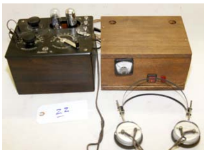
22. Radiola / III 1924; Tuned RF (TRF) receiver with power supply and headphones; working; has good WD-11 tubes.
