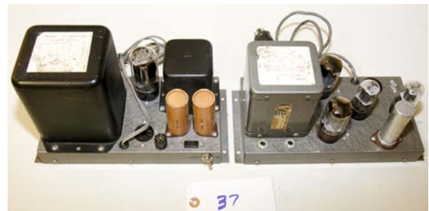
37. Heathkit / W-2M Circa 1951; power supply and mono amplifier; tested, working.
