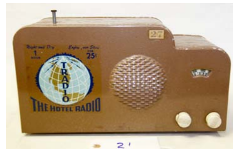
21. Tradio / L-U6 1947; AM band; coin operated hotel radio; has key; electronically restored.
