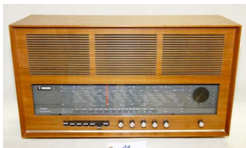
44. Saba / FD18 1966/67; AM/LW/SW/FM Stereo; electronically restored; has audio in; Bluetooth ready.
