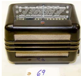
69. Philips / BD294 U 1949/50; AM/SW/LW; electronically restored.
