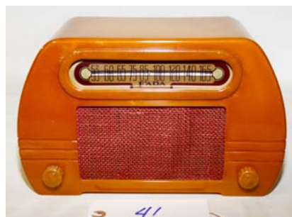
41. Fada / 652 Temple 1946; AM band; has Catalin case; electronically restored.
