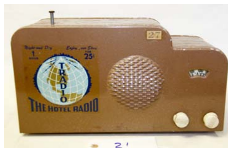
21. Tradio / L-U6 1947; AM band; coin operated hotel radio; has key.
