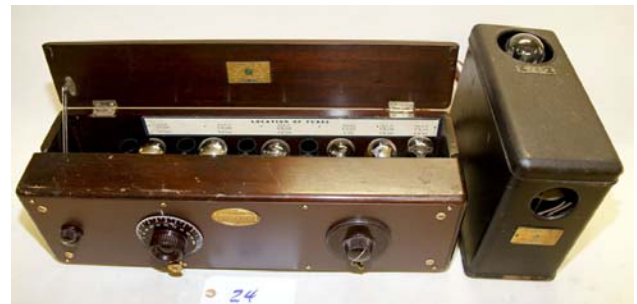
24. Atwater Kent / 36 1927; BC; has AK type Y power supply and Radiola UZ -325 speaker. Radio and power supply work.
