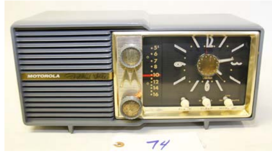
74. Motorola / 66C Golden Voice Circa 1956; BC, clock radio; electronically restored, on-off switch on rear panel; has audio in.
