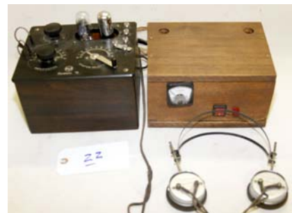
22. Radiola / III 1924; Tuned RF (TRF) receiver; has power supply and C. Brandes headphones.
