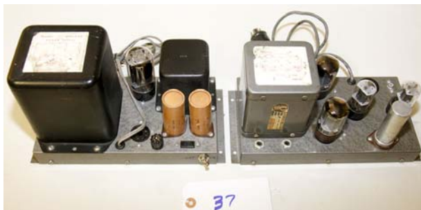
37. Heathkit / WA-1 Circa 1951; power supply and mono amplifier; tested, working
