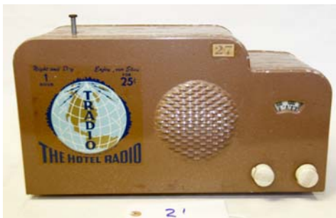
21. Tradio / L-U6 1947; Broadcast band; coin operated hotel radio; has key
