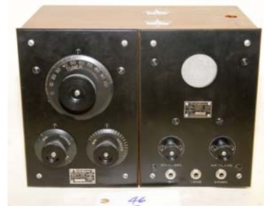
46. Westinghouse / RC (RA and DA combined) 1921; Tuned RF; Broadcast band
