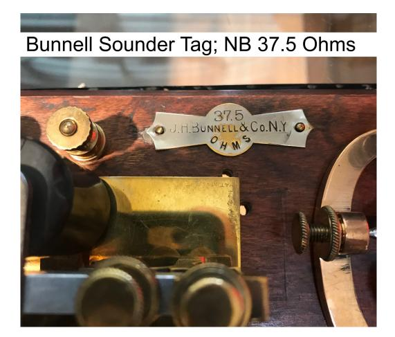
Note the 37.5 ohms figure. Failure to apply Ohms Law could burn out the sounder coils.
