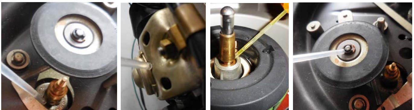
Lubricate the drive motor shaft, the rear bearing of the motor, and the idler wheel shaft. Clean the drive surfaces of the motor shaft and idler wheel with alcohol.
