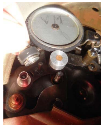
Turret drive lubrication with Moly grease.
