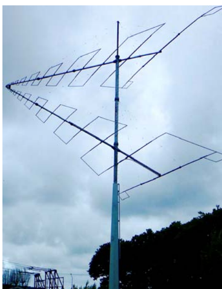
Fig. 17: SK6SAQ huge log periodic antenna.
