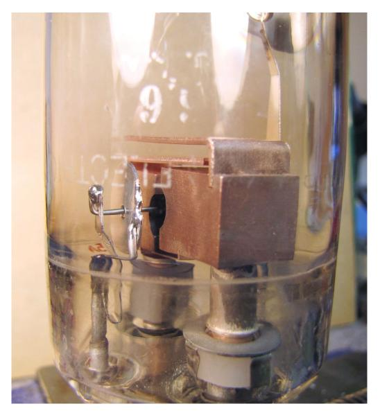
British National Valve Museum says of Fig. 2: "The [UK General Electric] GL5J29 is a two anode magnetron. The filament is visible as a rod passing through the circular hole formed by the two anodes. An output tuned circuit would be connected to the anodes with the DC power fed into a centre tap. The wide glass tube envelope is 47 mm in diameter and, excluding the base pins, is 150 mm tall. The base is a four pin special, with two large pins and two small pins."
