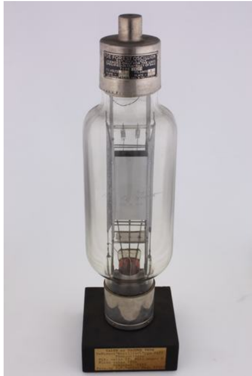
Item ST 15925 Electronic Valve - De Forest, Triode, Type 2Q15, circa 1921 https://collections.museumvictoria.com.au/items/369307
