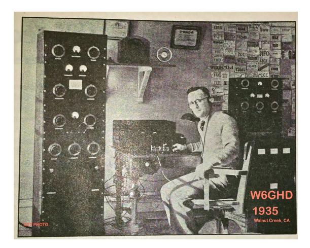
"The small rig on the file cabinet at the right in the photo is a low-power I60-meter 'phone, job using a pair of 46's to modulate a pair of 45's in the final. The r.f. plate input is about 40 watts. [160 meters, just under 2 MHz, was used as the local talk around band at the time]. The receiver will be recognized as a Hammerlund Comet Pro.
