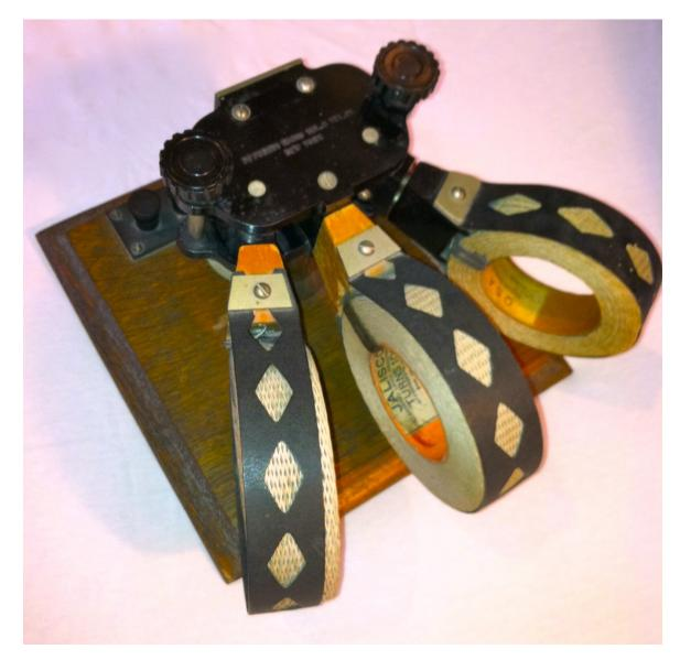
He also contributed a clever spring plug mounting to keep the coils mechanically stable during adjustment. In the photographs, one can see the top of the holder reading "De Forest Radio Tel. & Tel. Co. New York".
