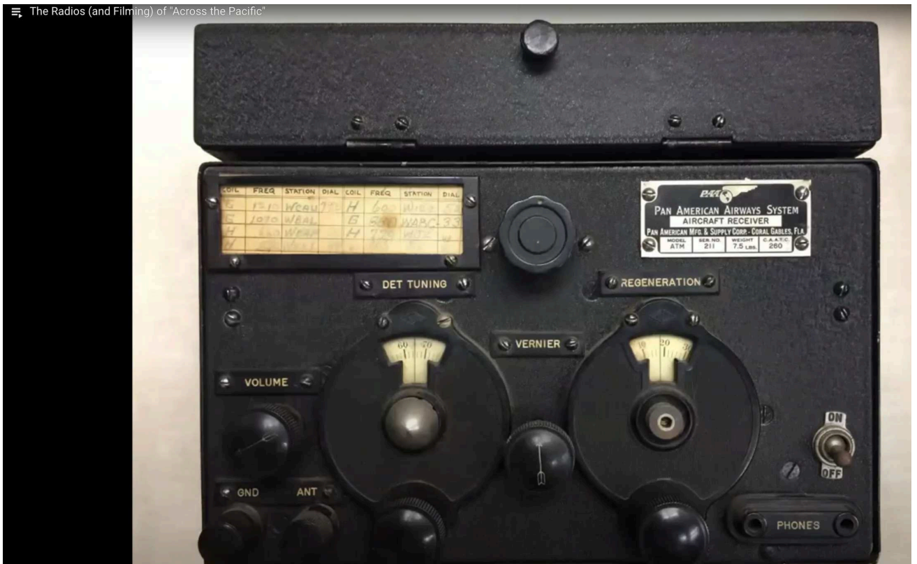
Pan Am aircraft model ATM receiver 1930s with coil box; AWA screenshot
