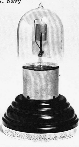
Moorhead amplifier tube SE-1444 used on the NC-3. #629 is also inscribed on the envelope
