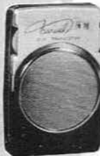
Model 6YR-21 6 TRANSISTOR Size: 3 1/2" x 2 1/2" x 1 1/2" Weight: 6.1 oz Battery: BL-006P, Eveready 216 or RCA VS 312, 9 V Speaker: 2" permanent dynamic
