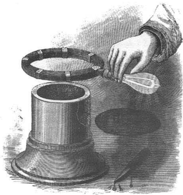
An early filament light bulb experiment with induction.
