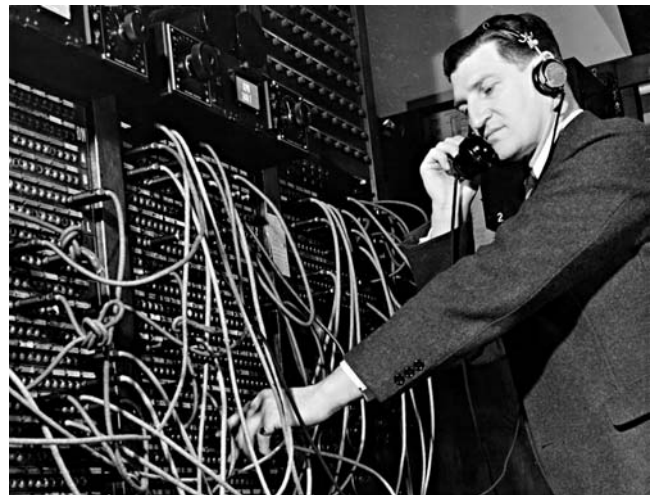
Left: Master Control at NBC in San Francisco, used from 1927 to 1942 with studio amplifiers, bridging equipment, power and testing equipment.
