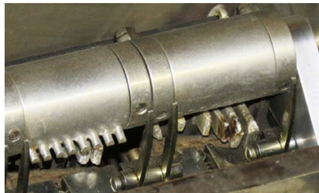
Solder was added to a reed to tune it to the desired frequency.
