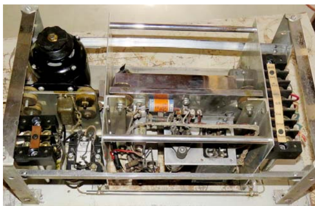
View of the underside 6C6 amplifier circuitry, motor, and power supply.
