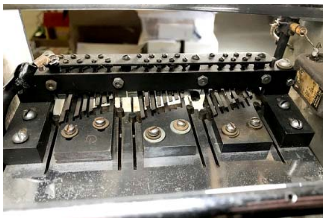
View of the capacitive pickup fingers and three vibrating reed combs. Note several reeds have been broken off.
