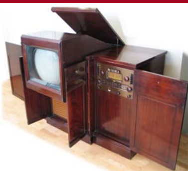
Figure 3 — DuMont RA-101 “Westminster” TV/radio/phonograph – an early form of an “entertainment center” in an enormous, yet stately cabinet. With the cabinet closed, the CRT faces upward inside the cabinet. Triggered by mercury switches in the doors, a motorized mechanism tilts the CRT into a horizontal position for viewing. To the left of the CRT (not visible) is a phonograph.
