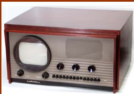
Figure 6 — Hallicrafters 505 TV. This set uses a 7JP4 CRT. The channel selector consists of a row of 13 buttons plus a 14 th which is for fine tuning.
