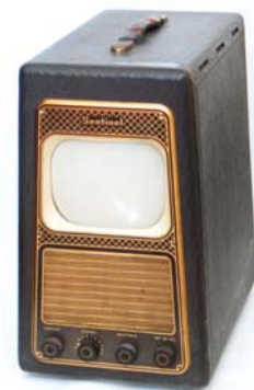
Figure 8 — Sentinel 400TV. Another inexpensive set from 1948 using a 7JP4 CRT. The upright “suitcase” design of this set is somewhat reminiscent of an oscilloscope design.
