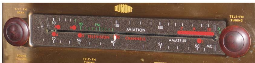
Figure 12 — The very unusual tuning dial of the DuMont RA-101 Westminster has a "wraparound" slide rule dial. The low frequency end of the dial begins with the VHF Low band in the lower right (marked with a red target for Channel 1).
