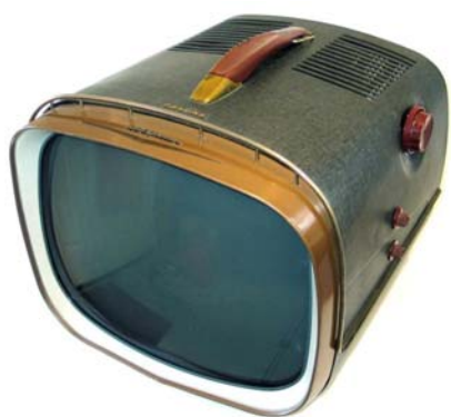
Figure 16 — RCA 14PD9030 portable from 1958. In addition to its distinctive styling somewhat reminiscent of 1950s automotive design, this set has a CRT with a tinted glass screen for higher contrast in a high level of ambient lighting.
