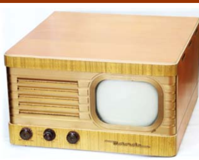
Figure 7 — Motorola VT-71. This was a very popular low-priced set using a 7JP4 CRT. It also came in a more common mahogany cabinet.
