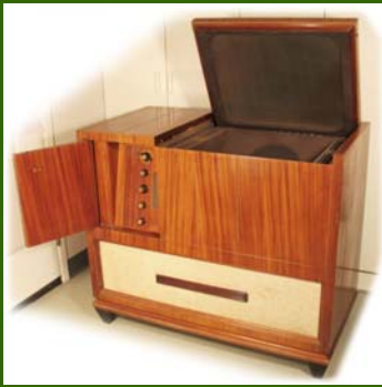
Figure 4 — Philco 48-2500 front projection set. Cabinet with lid open reveals projection screen on inside of lid. The far-right shows an actual picture produced by this set.
