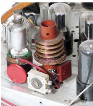
Figure 13 — Two approaches for generating high voltage for the CRT anode: (a) an RF transformer (left photo) and (b) a flyback transformer (right photo).
