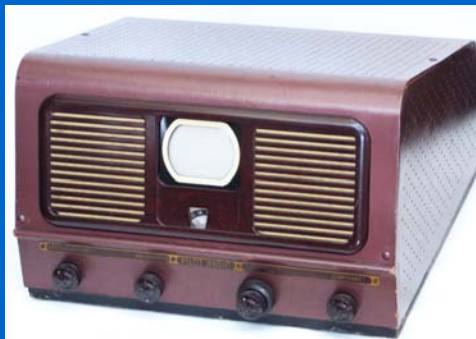
Figure 2 — Pilot TV-37 “Candid TV.” Its 3-inch screen made this the smallest TV of its time, with a price to match – only $99 in 1947. The Pilot’s chassis is no larger than a typical radio. Note the long slender 3KP4 electrostatically deflected CRT.
