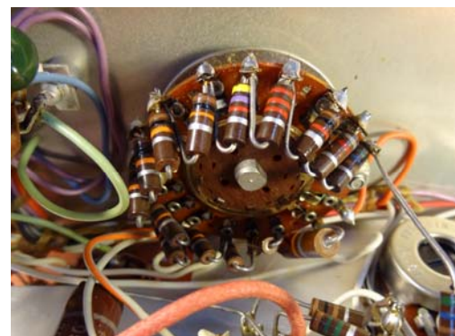
Poor solder joints on switch made during original kit assembly
