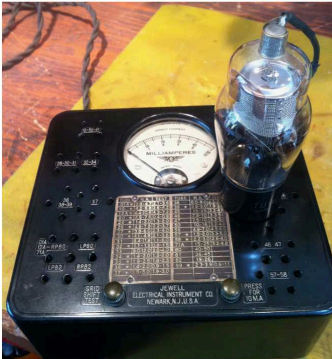
Type 24 tube as the DUT (device under test).
