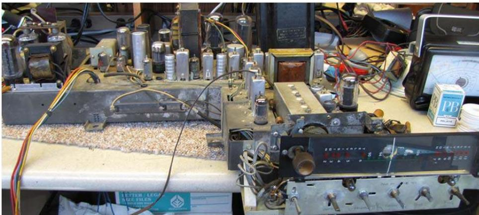
After the recapping and cleanup, both chassis were placed in the cabinet.
