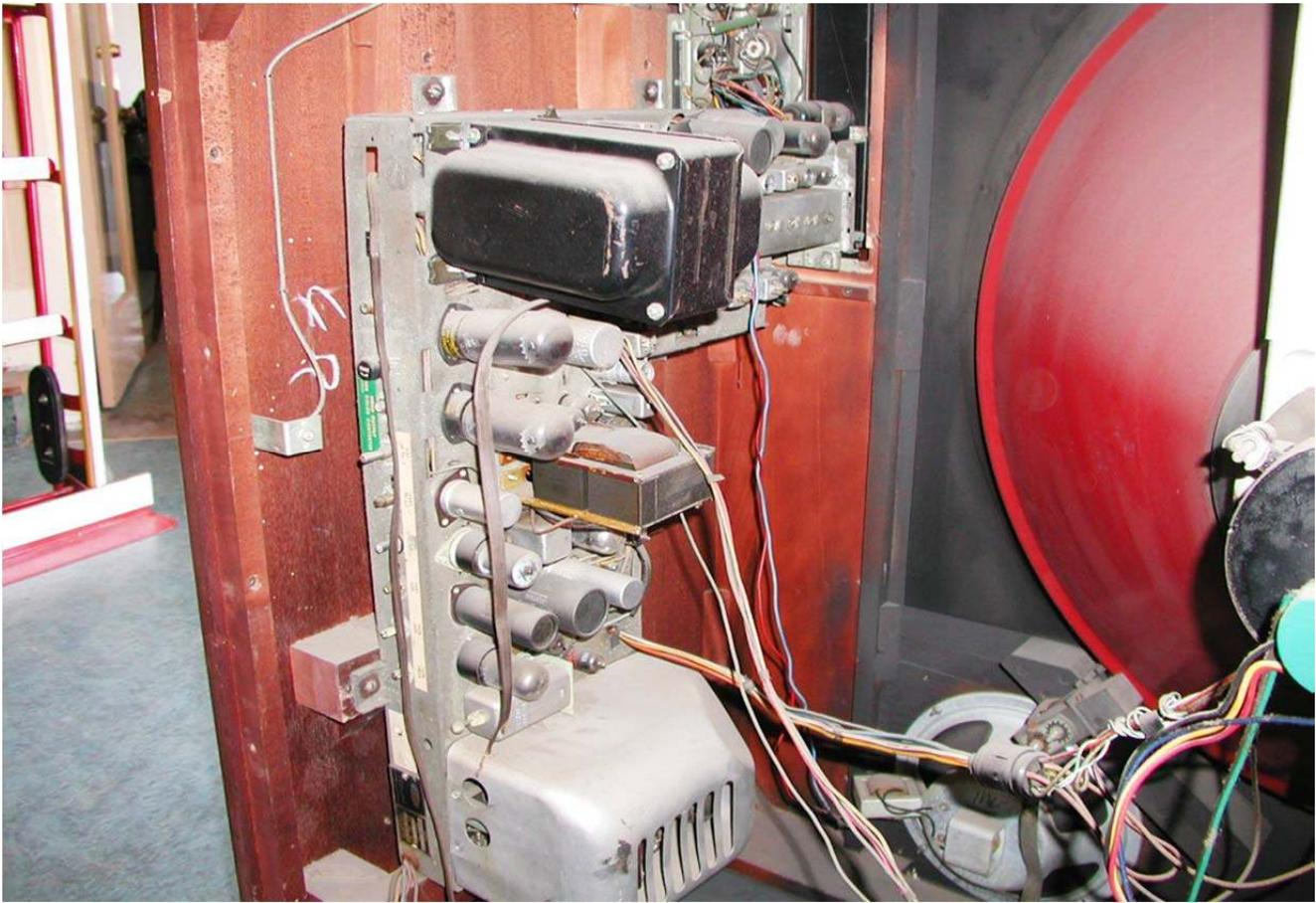
The RF/audio/deflection chassis is mounted on the side of the cabinet. The red cone of the CRT is mounted to its left.
