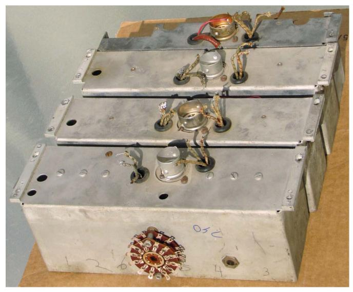
The miniature tube sockets are removed and the original octal sockets reinstalled. The original wafer switch at the front of the oscillator module has been lost. It controlled the IF gain separately for each band, as well as the RF AVC action for each band. New switch sections were found and configured to support these functions.
