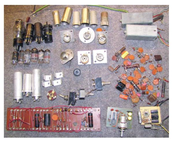
Six miniature tubes and their hardware, many passive components, a pegboard with several components from the modified IF/audio sections, an op-amp audio notch filter, and an IC-based crystal calibrator giving 100 and 500 kHz markers.
