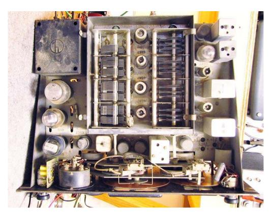
The first task was to strip the receiver and remove and replace the incorrect tube sockets, all the RF modules and the incorrect IF transformers.
