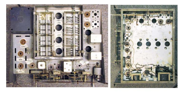
The receiver was then built back up, starting with the power supply and audio stages.
