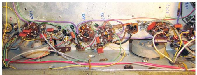
These are connected to the 6SC7 first audio stage, seen at the right behind the main tuning flywheel.
