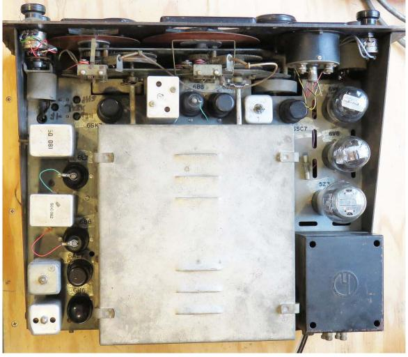
With the RF shield cover removed, the original metal octal tubes occupy the RF section, oscillator at the top, first RF stage at the bottom.
