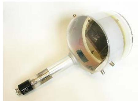
A lens focuses the scene on the mosaic, about the size of an index card, which consists of millions of small separate silver globules on an insulating mica substrate. The globules are treated with cesium, which renders them photosensitive, so they will emit photoelectrons when hit by light and thereby charge up. Behind the mica substrate is a full-size signal plate, connected to the video amplifier.
