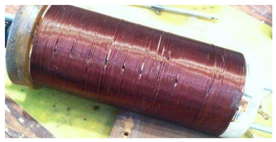
The Builder Pushed a "U" of Wire through the Coil Form after a Number of Turns and Held it in Place Inside with a Toothpick, and Soldered a Lead to each "U".
