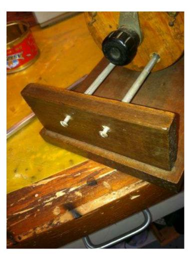
In the holes in the switch face are small copper tubes making electrical contact with the rods. The rotor connects to one tube (and hence its rod) and the near end of the coil to the other tube and rod.
