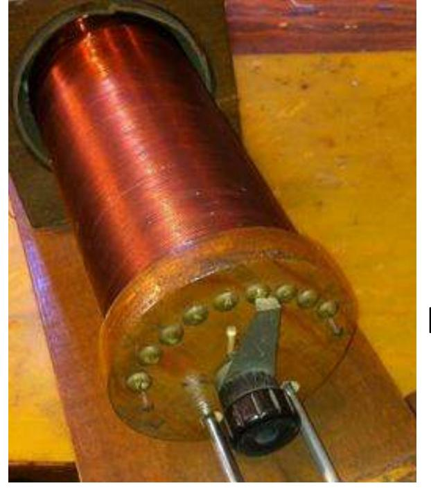
Inner Coil Re-Inserted In Outer Coil
