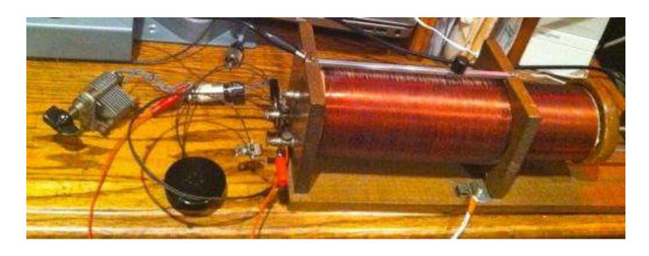
The Best Result so far: KCBS at a good volume (recorded); slider ¾ down big coil, inner coil ½ in, variable capacitor at 70 pF ±.
