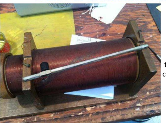
The antenna and ground connect to the big coil with the slider; the inner coil slides in and out with more or less of it switched in.
