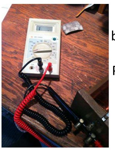
Also, no continuity between the big Coil "Earth" Binding Post and the big Coil -- a bad Connection inside the Coil.
