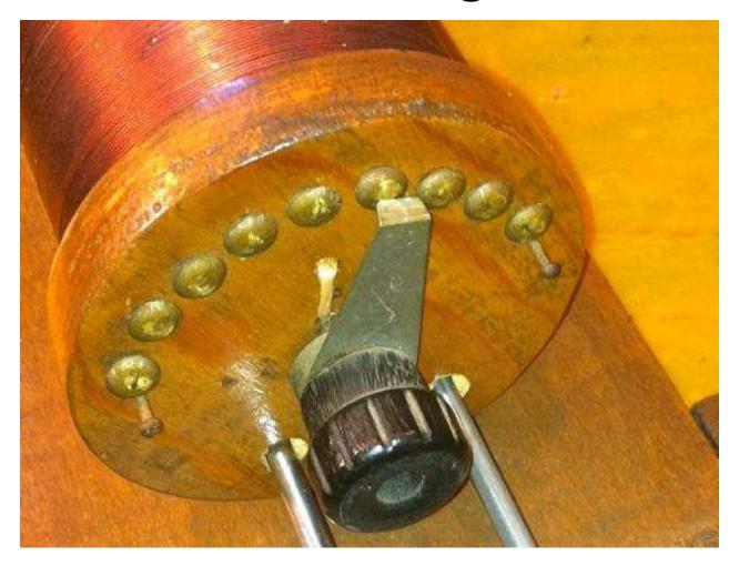
The Switch Points are Brass Tacks, the Stops are Nails.
