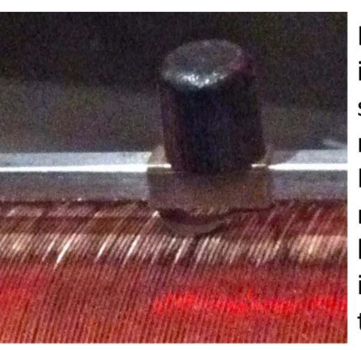
KCBS loudest at ½ big coil, inner coil about ½ in, and series cap tuned for maximum; KFBK good with inner coil minimally inserted, slider left for maximal inductance, series cap tuned for maximum.
