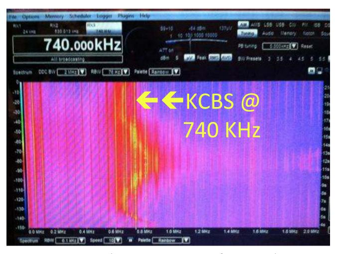
KCBS Maximum 4 mv  $\pm$ , but movement of one inch  $\pm$  can Minimize Audibility (100 microvolts  $\pm$ ); Variable Capacitor has no Effect.
