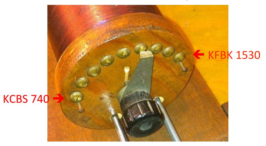
Inner Coil ½ in, Slider on Outer Coil ¾ over to the right (fewer turns engaged).
