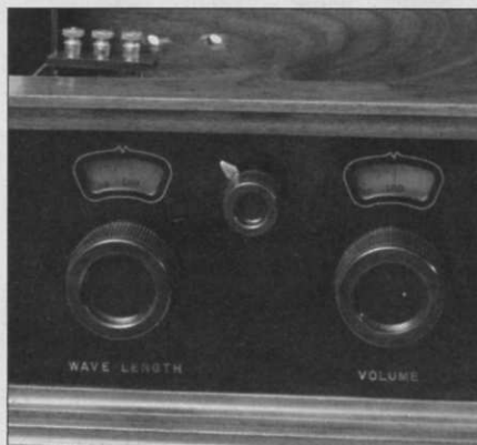
Figure 5 — This is the left side of the superdyne’s front panel. Note that the volume control adjusts the variometer. The more negative feedback, the lower the gain in the stages. [Steven Johannessen, photo]
