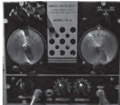
Figure 20 Abbott TR-4 Transceiver for 2&½ meters, 112 MHz of the type used in WERS in San Francisco (author's collection).
