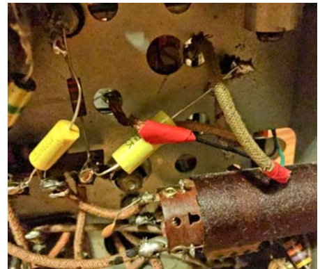
Connection of capacitor sense circuit to variable tuning capacitor.
