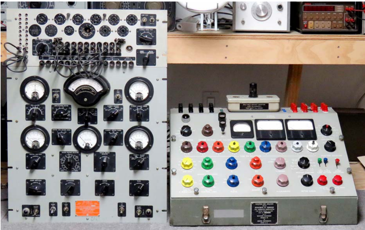
Laboratory grade tube testers: AN/USM-31 (Weston 686-C9) on the left, and Daystrom/Weston CA-1630 on the right.
