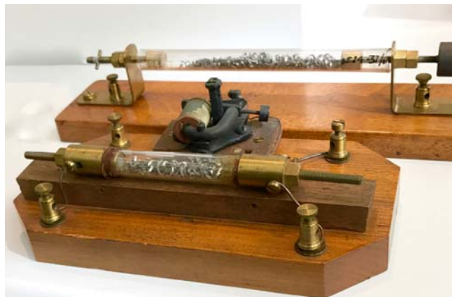
Fig. 20: Coherer using iron filings.
