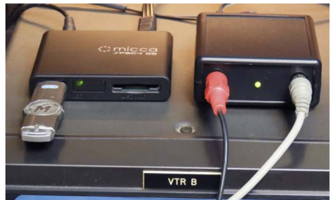
Left is the Micca video generator. Right is the Aurora SCM video format converter.
