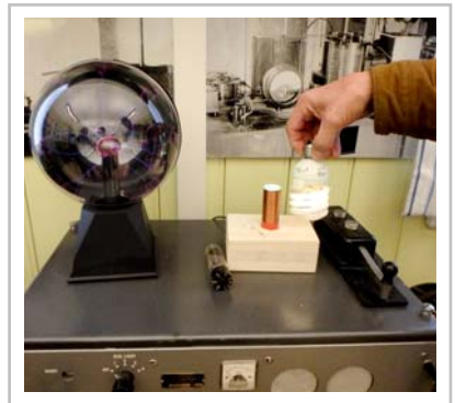
Fig. 19: Miniature Tesla coil lighting a florescent lamp.
