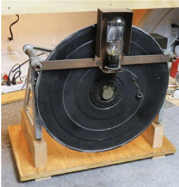
The Nipkow disk mounted in a temporary frame.
