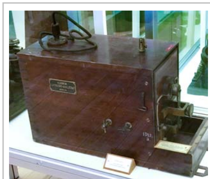
Fig. 3: Slaby-Arco spark coil. Below is the label.
