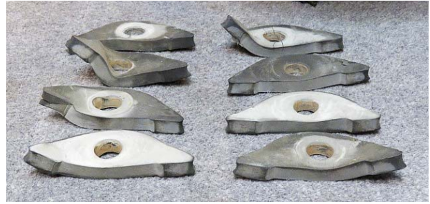
The original rubber isolation mounts.
