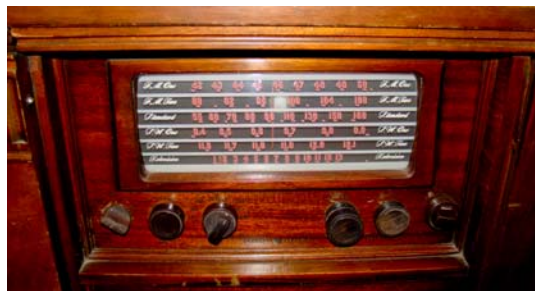
Fig. 16: The GE 901 projection set (1946). The dial includes both pre-war and post-war FM bands — very unusual.
