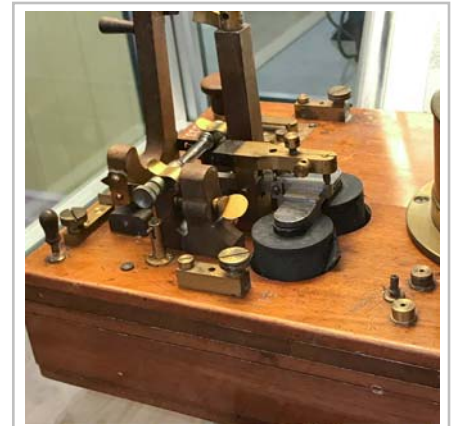
Fig. 5: Slaby-Arco coherer. Below is the label.
