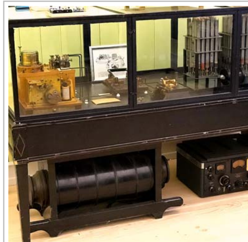
Fig. 7: Large Ruhmkorff coil on the floor and spark receiver in the case.
