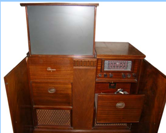
Fig. 16: The GE 901 projection set (1946). The dial includes both pre-war and post-war FM bands — very unusual.
