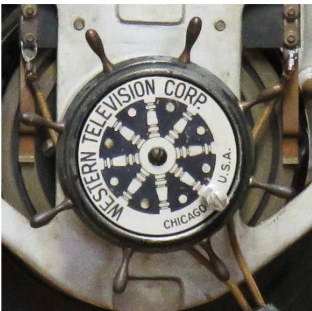
This wheel is turned by the user to initially start the motor. Then its used to frame the image.
