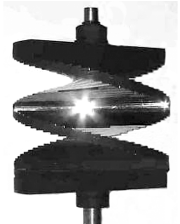
Fig. 1: A mirror screw is a stack of thin narrow metal blades or slats that have been polished on their edge to a mirror finish and mounted on a shaft. Source: Peter Yanczer
