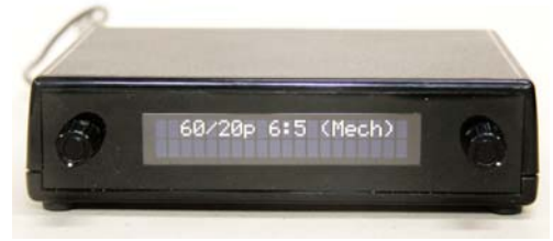
Fig. 10: Aurora World Converter (WC01) video standards converter.
