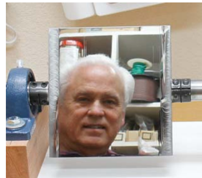
Fig. 7: The mirror screw after polishing and before the alignment of the slats. Perhaps this is the first mirror screw selfie.
