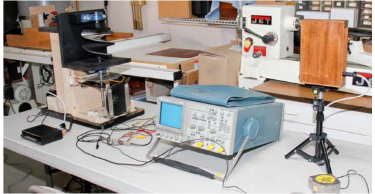
Fig. 13: Test setup with mirror screw set on the left and light source on a small tripod to the right. The oscilloscope was there to assess sync pulses.
