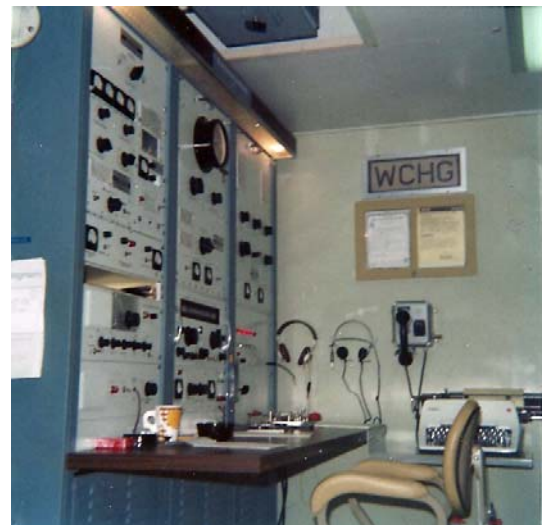
Fig. 5: Hughes Glomar Explorer WCHG transmitters: Collins 208U-3 (3 KW), and Communications Associates Inc. Transceiver (1 KW).
