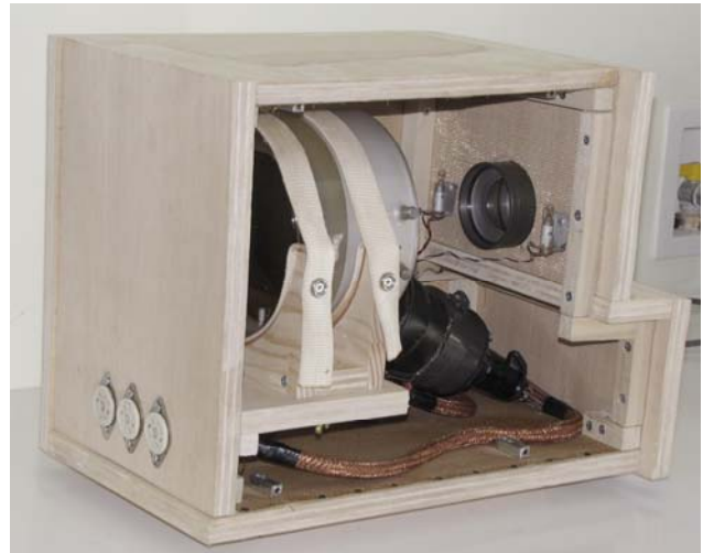
Iconoscope installed in the case.
