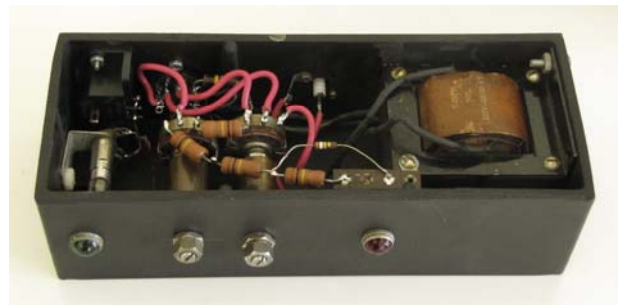
Box showing the resistive divider and two potentiometers for focus and beam current.
