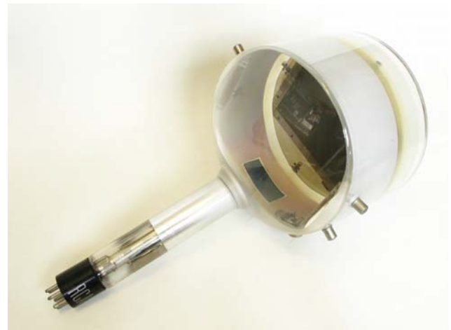
The RCA 1850A iconoscope tube.
