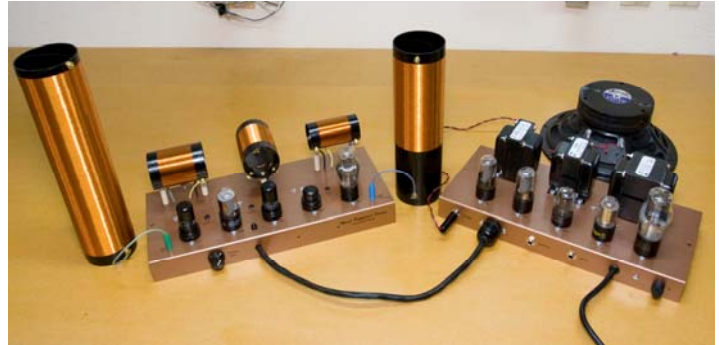
The Mark Keppinger designed Theremin. Power chassis right., Oscillator chassis left. Pitch coil far left, volume coil center.
