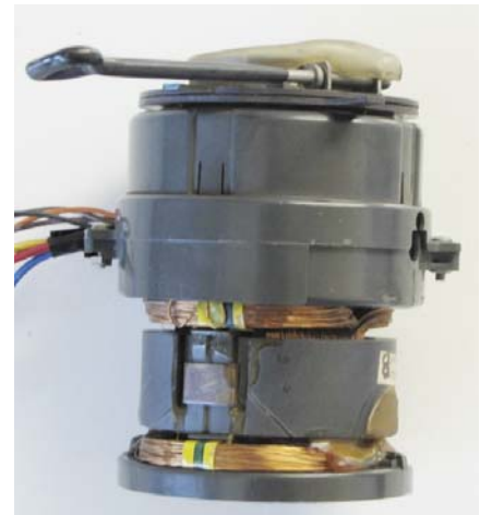
Yoke repurposed for the iconoscope.
