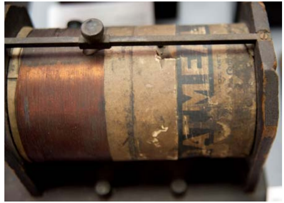
Basic crystal set homemade coil.
