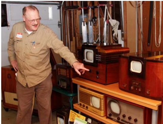
Nat Pendelton demonstrates his RCA TT-5, a pre WWII set. This set had no audio amp, audio has to be played through the radio sitting on the table left (under his arm). On the right is a General Electric HM-171, another pre WWII set. Both sets are from 1939 and quite rare.
