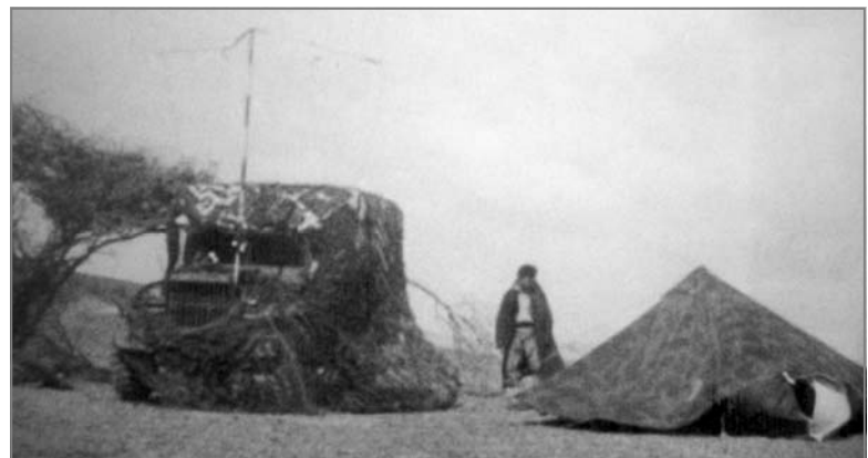
Fig. 8: An Israeli mobile monitoring station at a front in 1948; note the antenna mast at the front of the truck [2].
