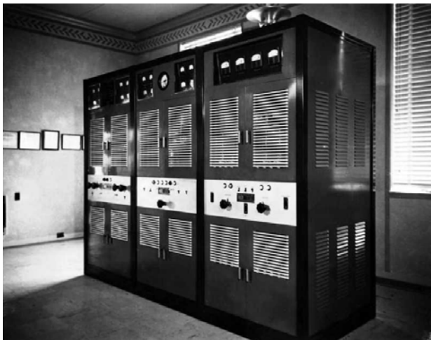
Fig. 23: RCA 5-C Transmitter in the new art deco building.
