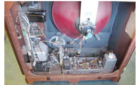
The RCA CTC-12 chassis on the bottom, replacing the missing HV chassis.
