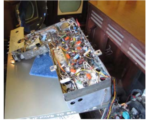
The RF chassis on a cart behind the cabinet, hooked up for checking its operation.
