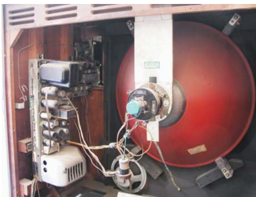
The interior showing the 30" CRT and the RF and deflection chassis. The second LV and HV chassis is missing from the bottom of the cabinet.
