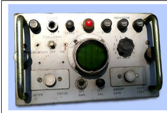
Fig. 5: This is the display unit of a World War Two IFF (Identification Friend or Foe) equipment. The scope showed a vertical trace displaying the return signal from an aircraft's transponder. Note, top left, a control by which a signal could be sent to an aircraft as a "challenge." (Bart Lee collection and photo).
