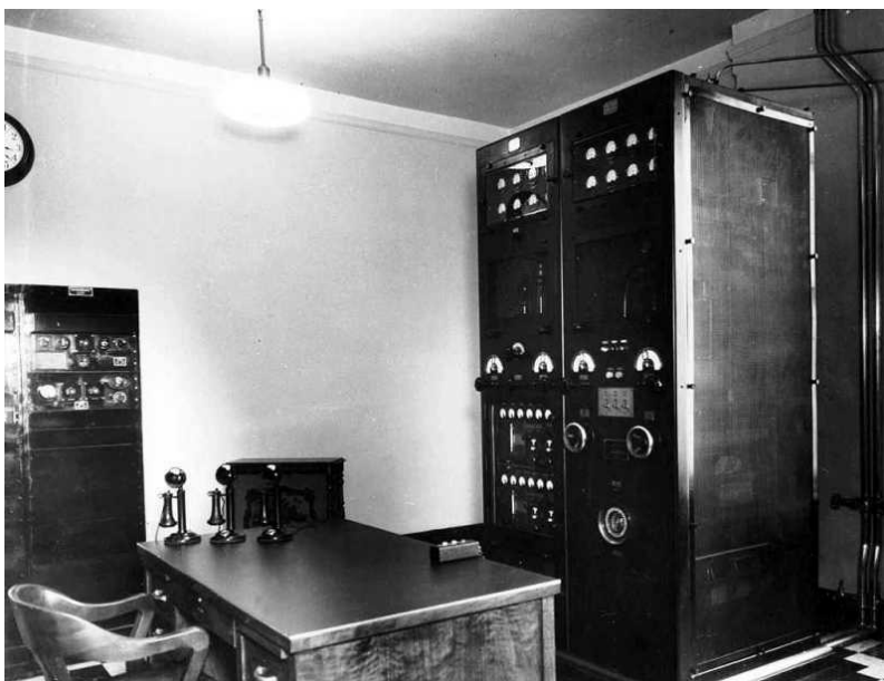
Fig.13: The RCA 1001-B transmitter at the Hotel Whitcomb (circa 1930).
