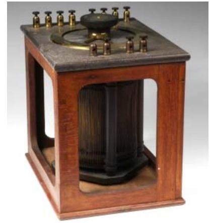
Fig. 4: Marconi Direction Finder, c.1916. Designed to detect positions of wireless stations. Source: Wireless World, Marconi and the Making Of Radio.
