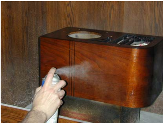
Figure 17: Spraying the clear coat.
