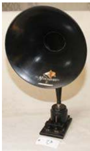
73. Magnavox / R3 $150 1920s; horn speaker with driver; passes click test
