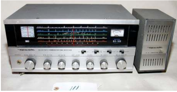
111. Realistic / DX-160 $80 1975; 5-band AM, SSB communications receiver (BC/SW/LW); has speaker; works
