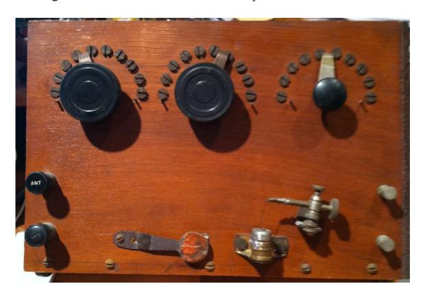
This set seems to be a buzzer transmitter and crystal receiver. Note the homemade key on the front.
