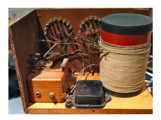
Tom Perrara has a nice web page that deals with buzzer sparks. <a href="http://w1tp.com/perwirls.htm">http://w1tp.com/perwirls.htm</a>. That's his illustration of a key buzzer. He says that this code practice set, with a wire attached to the buzzer, worked as a transmitter.
