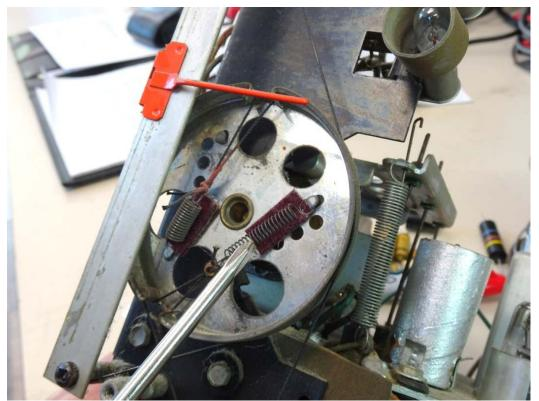
spring from main pulley and reattaching it further up the coil spring (see photo at right). Decades ago, some restorers used cloth line to replace broken dial string cords, and these usually deteriorate with time and break. Make sure to use nylon line for long life.
