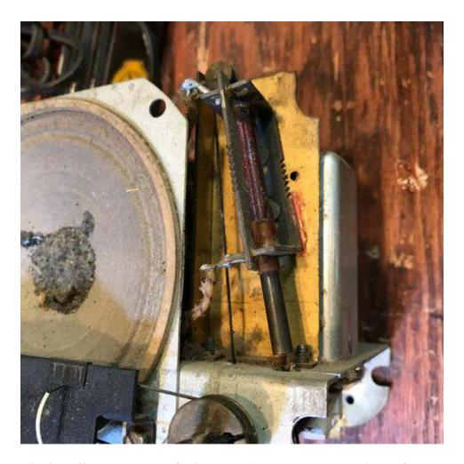
This is "permeability" tuning of the inductance with a ferrite core or slug.
